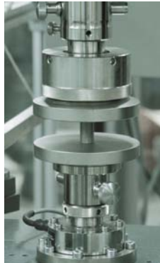
Picture 1.6: Testing of the compressive strength of iglide® plain bearings
