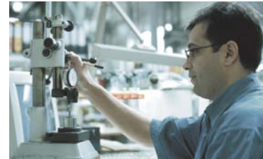
Picture 1.19: Measurement of the inner diameter of a pressfit plain bearing
