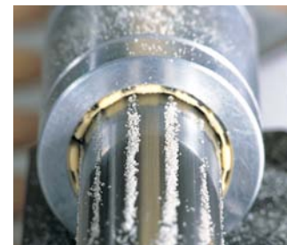
Picture 1.16: High wear resistance: plain bearing in contact with sand
