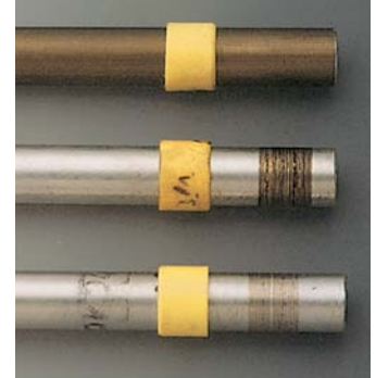
Picture 1.17: Wear experiments with aluminum shafts
