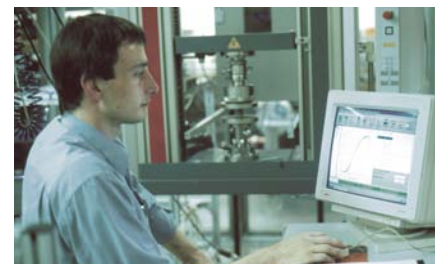
Picture 1.9: Testing the properties of plastic bearings
