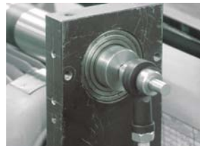
Picture 1.8: Determining the maximum surface speeds of an igubal rod end bearing at high rotational speeds
