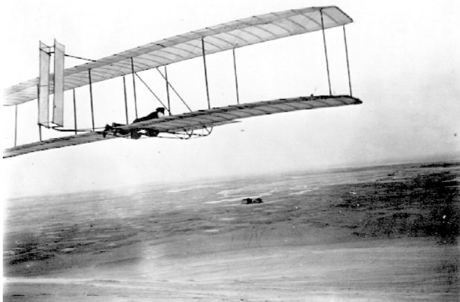
Figure 37. Testing the two-surface rudder on the 1902 glider in October 1903.
