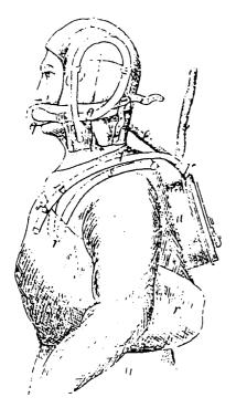
This drawing from Newton's patent specification shows the demand valve on the diver's back and the "stab jacket"on his chest and under his arms with the looped exhaust tube by his head.
