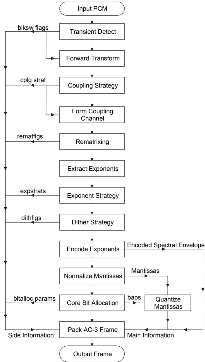
**Figure 8.1.** Flow diagram of the encoding process.
