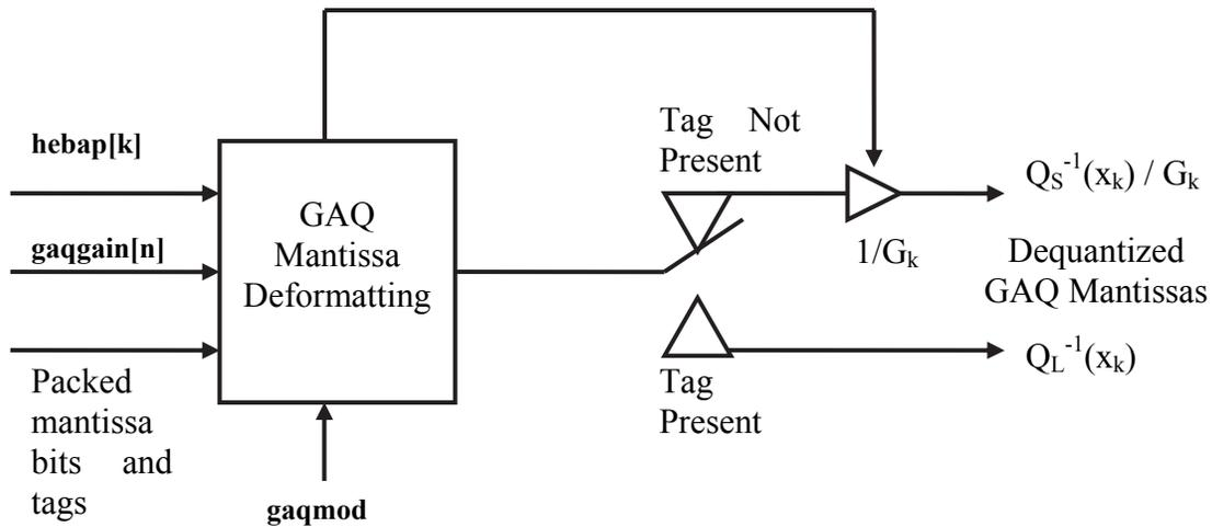
**Figure E3.1** Flow diagram for GAQ mantissa dequantization.
