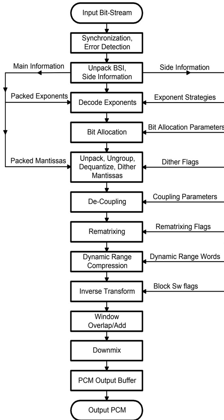
**Figure 6.1** Flow diagram of the decoding process.
