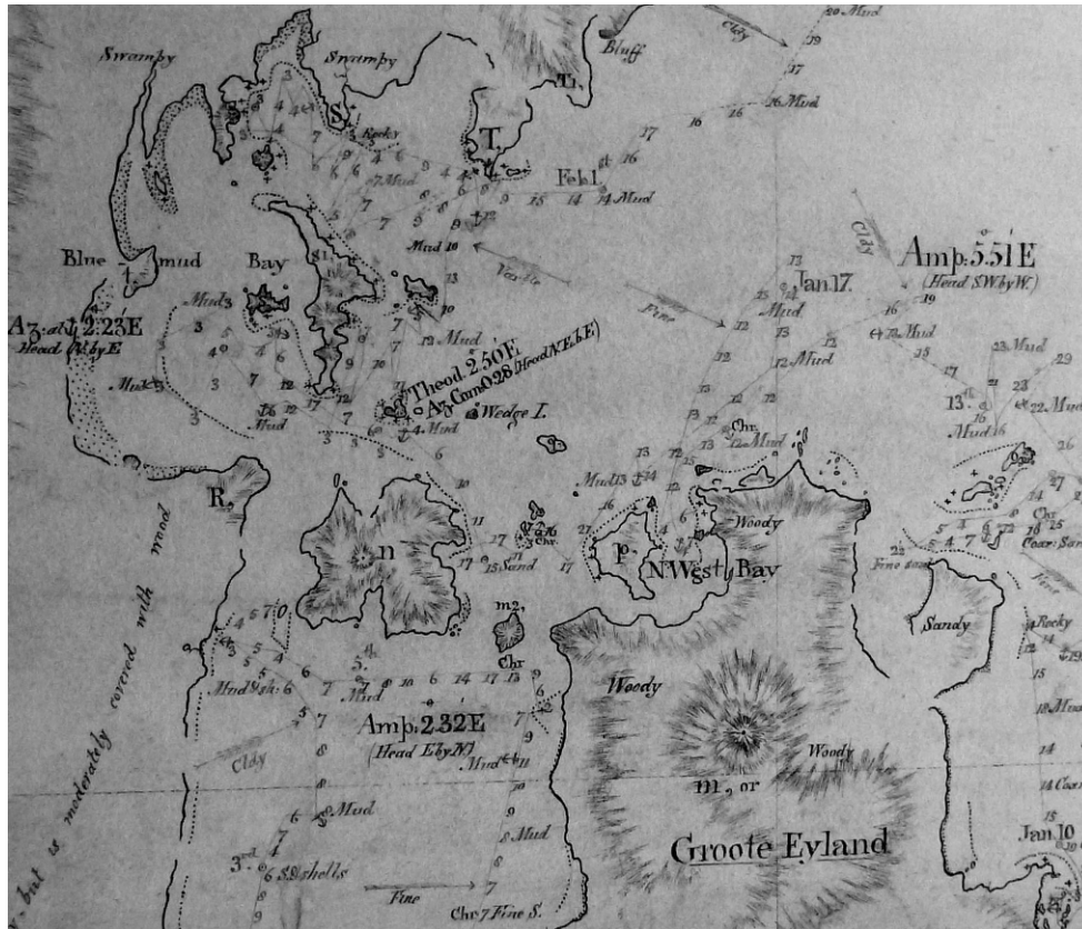
Figure 1: An example of Matthew Flinders's working sheet, with letters from m to T to label the islands and geographical features surveyed during the Investigator voyage. Source: Part of the North Coast of Terra Australis from sheets N o 1, 2 & 3 , by M. Flinders Commr of HM Ship Investigator & Schooner Cumberland Mauritius Jan 18 1804, TNA ADM 352/548.
