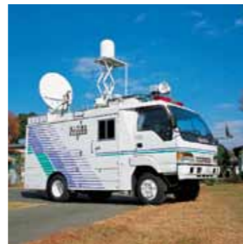
Vehicle equipped with satellite communication system
