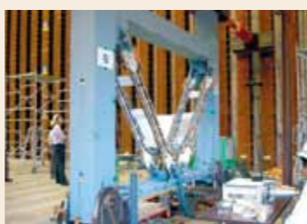
Model experiment using a 1/6-scale model of braces for restraining buckling
