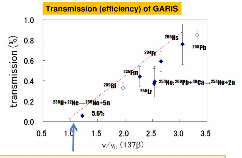
Small efficiency because of slowness of the ion multiple scattering with target atoms  $$\sim 30\%$$  multiple scattering with buffer gas atoms  $$\sim 17\%$
