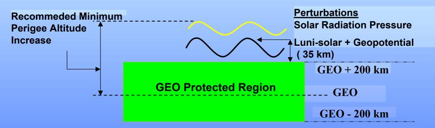
Re-orbit distance was determined as the sum of the upper side of GEO protected region (200 km), the maximum descent of a re-orbited space system due to luni-solar & geopotential perturbations (35 km) and solar radiation pressure.
