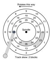
Figure 37.4: Three Tracks: Track Skew Of 2
