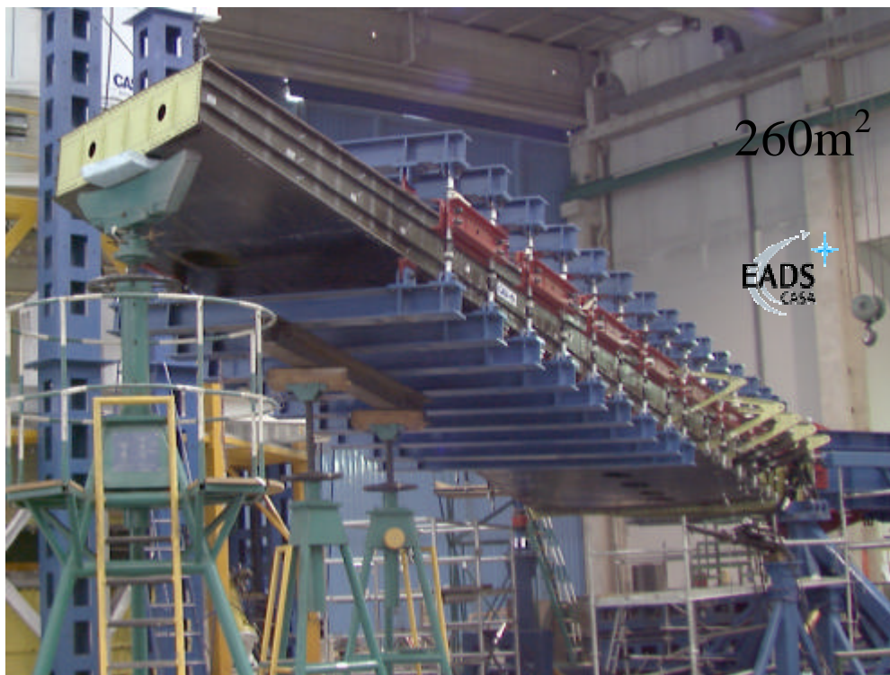
Figure 8: A380 Horizontal Tailplane composite torsion box demonstrator (Automated Tape Laying)
