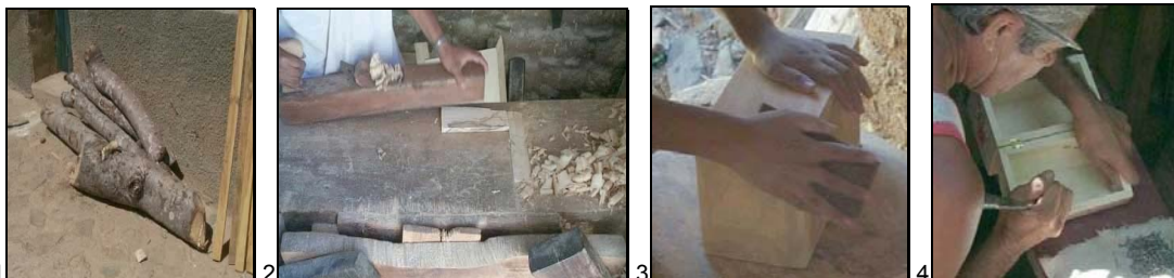
1 Pieces of cut wood left to dry (1); wooden parts are sawed to size and planed (2); building and planing a chest (3); fitting the locks and hinges (4) (photos: worldexperience.com ).
