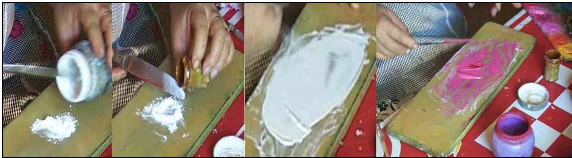
Preparation of lacquer: tesicalte , adding oil to the powder, the lacquer mixture and the lacquer after a pigment has been added. (foto's: worldexperience.com ).
