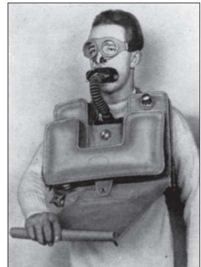
Figure 1-10. Original Davis Submerged Escape Apparatus.
