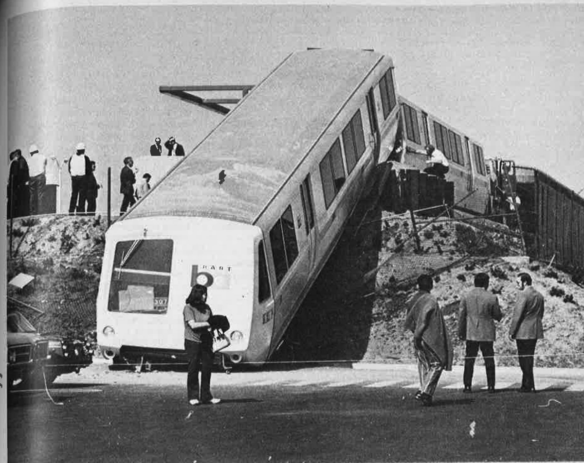
The incident of October 2, 1972. Lead car of BART train overshot the terminal station at Fremont and came to rest on a sand embankment following a failure in the ATC system. (Photo courtesy Lonnie Wilson, Oakland Tribune .)
