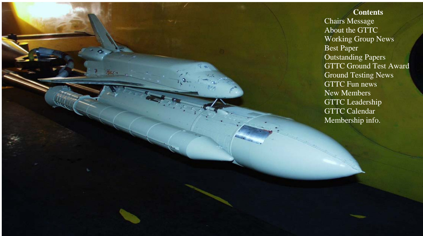
Wind tunnel model of the orbiter installed in the NASA Ames 9x7 SWT
