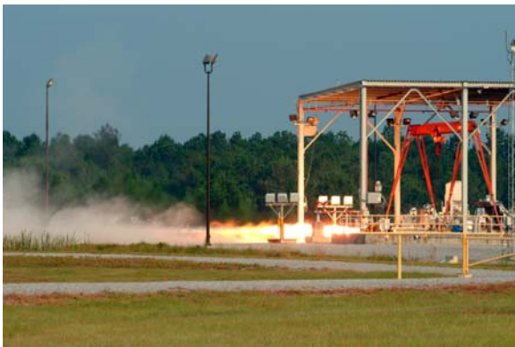
Paraffin-Fuel Rocket Motor Tested at Stennis Space Center
