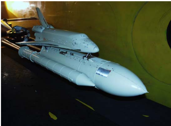
Wind tunnel model of the orbiter installed in the NASA Ames 9x7 SWT
