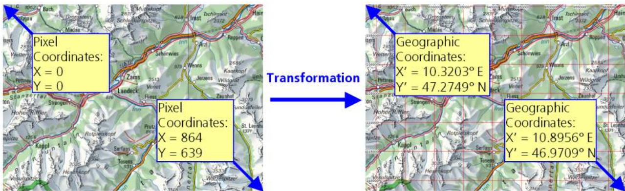
Figure 22: Raster map with pixel coordinates X,Y (left) and vector map with geographic coordinates X', Y' (right)
