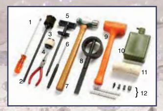
Flat tip 6,5 X 200 screwdriver Cleaning Rod extention with Brush Barrel Swop Long nose Plier Cleaning Rod 6,5mm Pin Punch Bolpin Hamer Barrel Spanner 18oz Mallet (510g)
