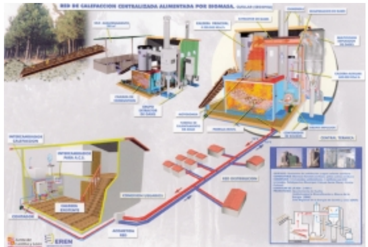
A centralised water and heating system with the use of forest residues as a raw material in Cuellar, (Province of Segovia, Castilla y León Region, Spain). Biomass is used as fuel for a steam power plant in which water is heated for its later distribution to end-users through a preinsulated double pipe-line system. Sources: EREN (Spain)
