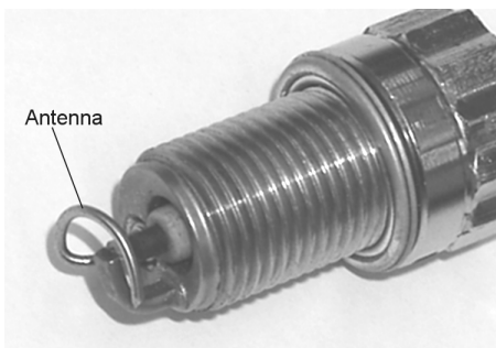
Fig. 10 Prototype of spark plug having a microwave antenna.
