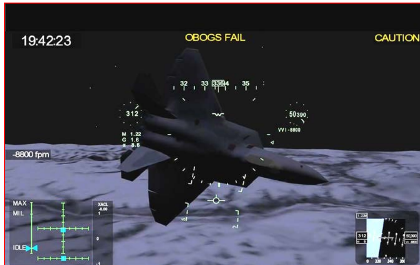
Figure 2 19:42:23L -- MA parameters at assertion of OBOGS FAIL caution ICAW. (Tabs EE-3, Z-10)
