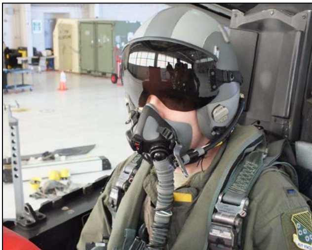
Figure 13 -- F-22A Pilot wearing helmet with left mask bayonet disconnected. (Second Addendum Tab C-4)
