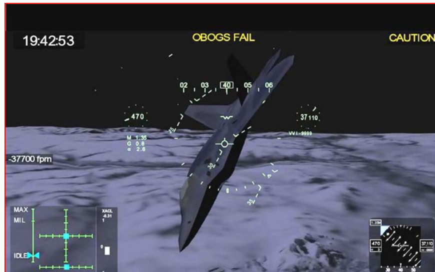
Figure 4 19:42:53L -- MA parameters after 8 seconds of zero MP inputs to stick, pedals, or throttles. (Tabs EE-3, Z-10)
