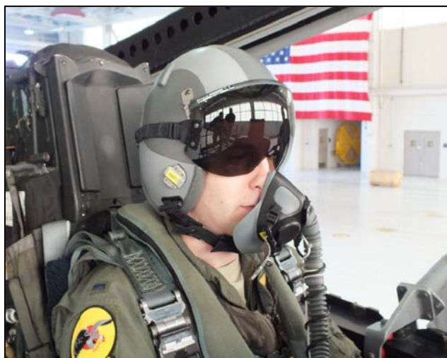
Figure 14 -- F-22A Pilot wearing helmet with right mask bayonet disconnected. (Second Addendum Tab C-6)
