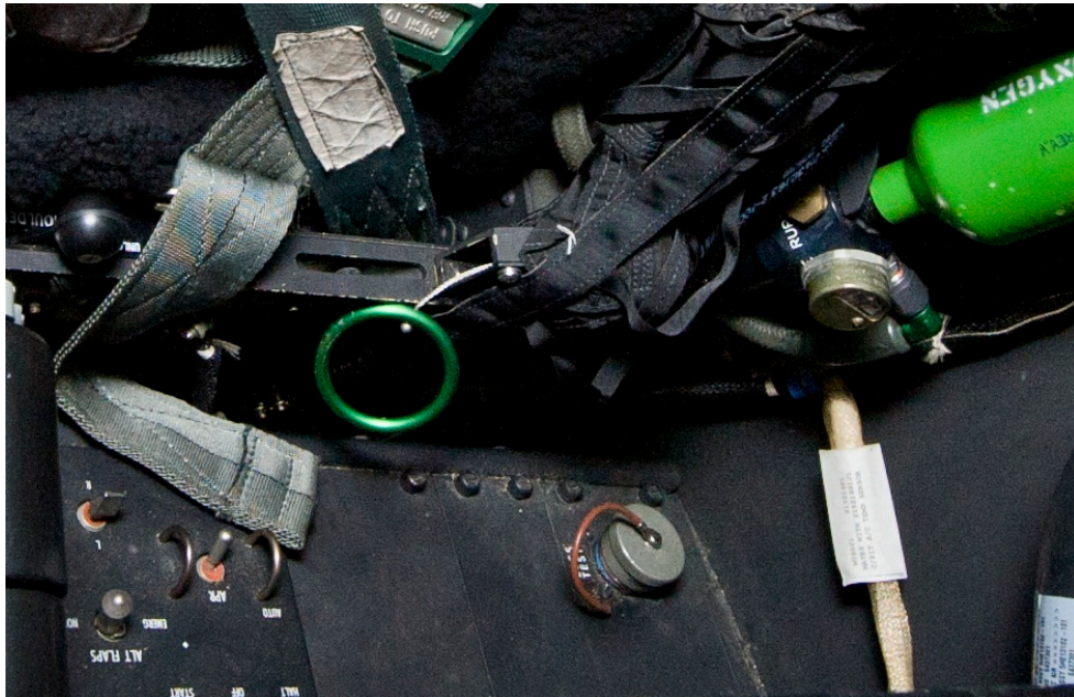
Figure 17 -- Manual EOS activation ring fallen below lip of seat. (Tabs Z-8, CC-5)
