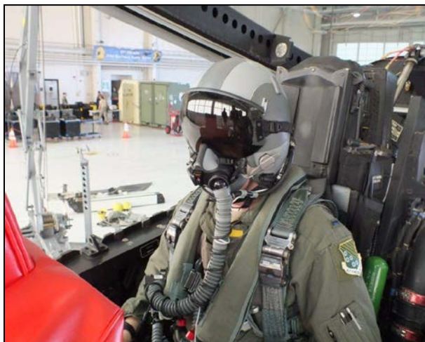
Figure 12 -- F-22A Pilot wearing helmet with mask up and secured. (Second Addendum Tab C-4)
