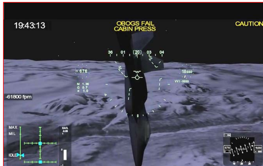
Figure 6 19:43:13L -- MA parameters at assertion of CABIN PRESS caution ICAW. (Tabs EE-3, Z-10)
