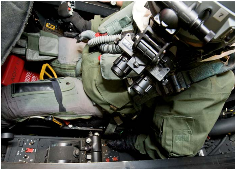
Figure 16 -- Pilot advisor pulling EOS activation ring. NVGs interfering with EOS activation ring visualization. (Tabs Z-7, CC-5)
