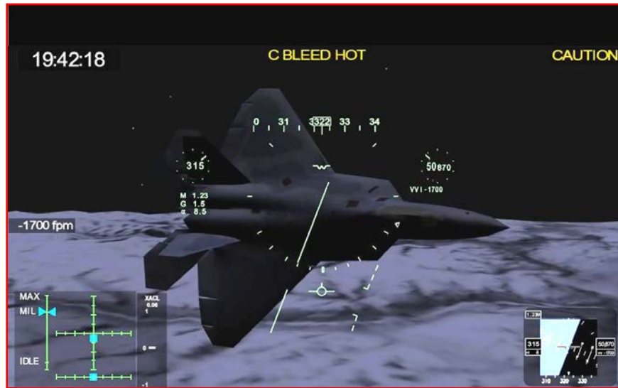
Figure 1 19:42:18L -- MA parameters at assertion of C BLEED HOT caution ICAW. (Tab EE-3) (See Tab Z-10 for a diagram explaining the symbology in the Figures.)
