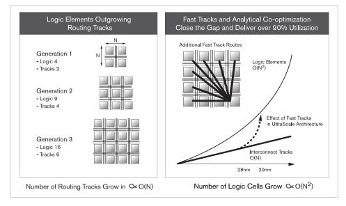
result is an exponential increase in the amount of data the UltraScale Architecture can manage, as shown above in the diagram on the right.
