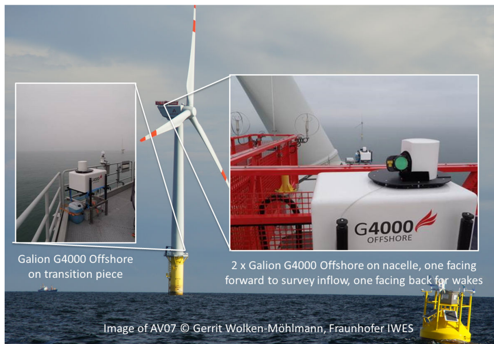
Figure 1: Alpha Ventus Offshore Wind Farm Wind Turbine #7 with scanning lidars installed
