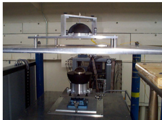
Fig. 4 Final configuration of the ^{237}\text{Np} /HEU experiment.
