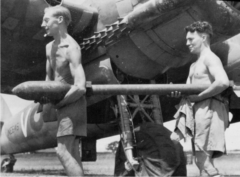
A 3-inch RP with a 60 lb warhead about to be loaded onto a Beaufighter in India.
