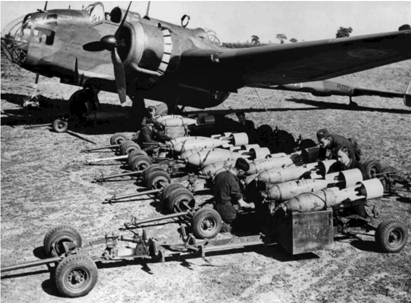
Compare and contrast: above, the Hampden of 1939 with a typical load of GP bombs and, below, the Lancaster of 1945 with up to 14,000 lbs of HC and MC bombs.
