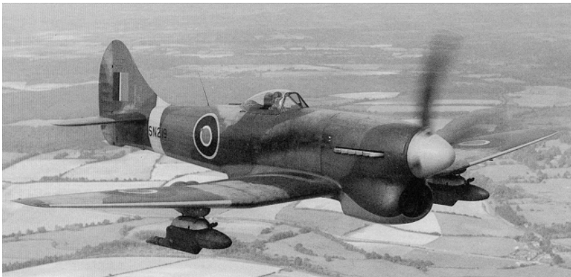
Trial installation of an M10 Smoke Tank on a Tempest V.
