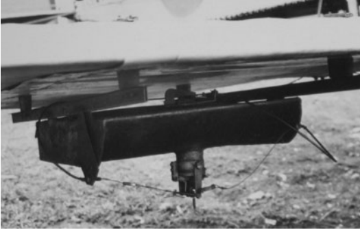
A spray tank, similar to those used by the FAA, fitted to a Bristol Fighter engaged on trials work.
