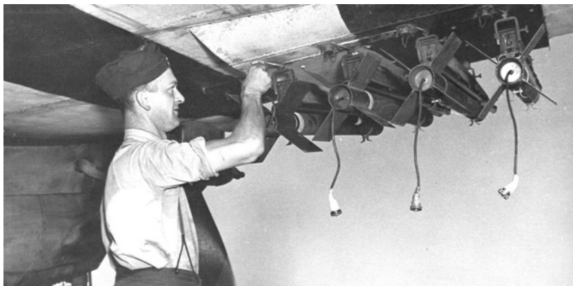
The 'pigtails' of a load of 3-inch RPs with 25 lb warheads being connected up on a Coastal Command Beaufighter.
