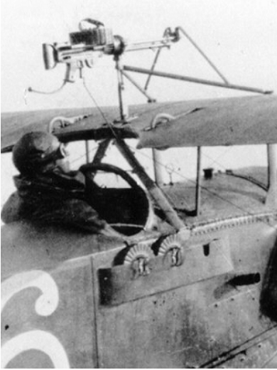
Nieuport with an upper wing mounting (left) and the much handier Foster mounting of a Lewis gun on an SE5a.
