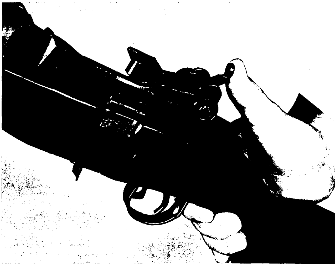
Figure 47. Adjusting sight tension.
