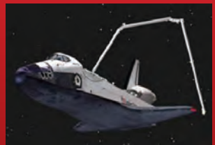
Astronaut Naoko Yamazaki used the Orbiter Boom Sensor System (OBSS) as an extension to the Discovery's robotic arm—the Shuttle Remote Manipulator System (SRMS)—to check for any damage to the spacecraft's body. This inspection was an important operation to ensure that there were no problems with the shuttle's Thermal Protection System (TPS) during re-entry into the Earth's atmosphere.
