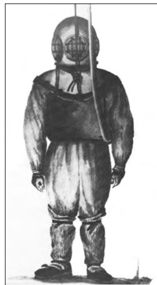
Figure 1-5. Siebe's First Enclosed Diving Dress and Helmet.
