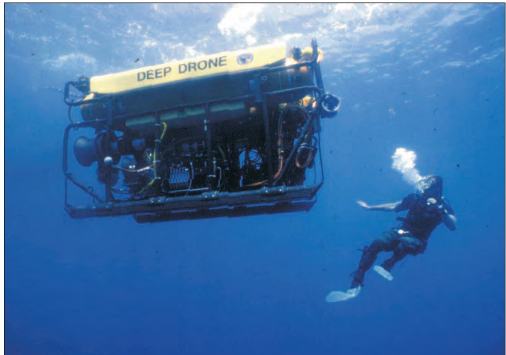
Figure 13-2. Remotely Operated Vehicle (ROV) Deep Drone.
