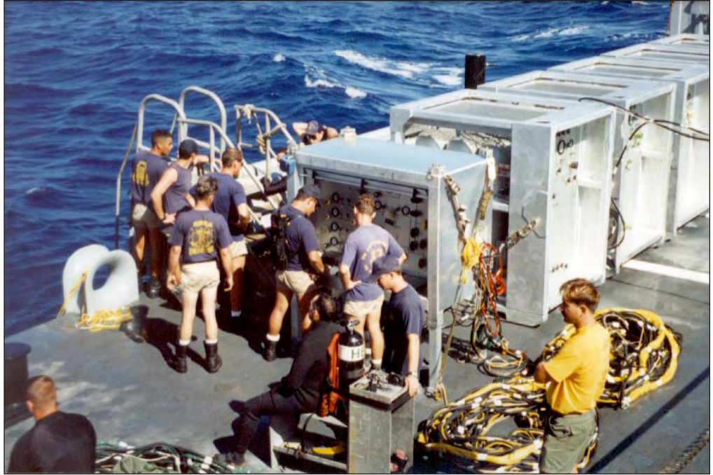
Figure 13-5. FADS III Mixed Gas System (FMGS).
