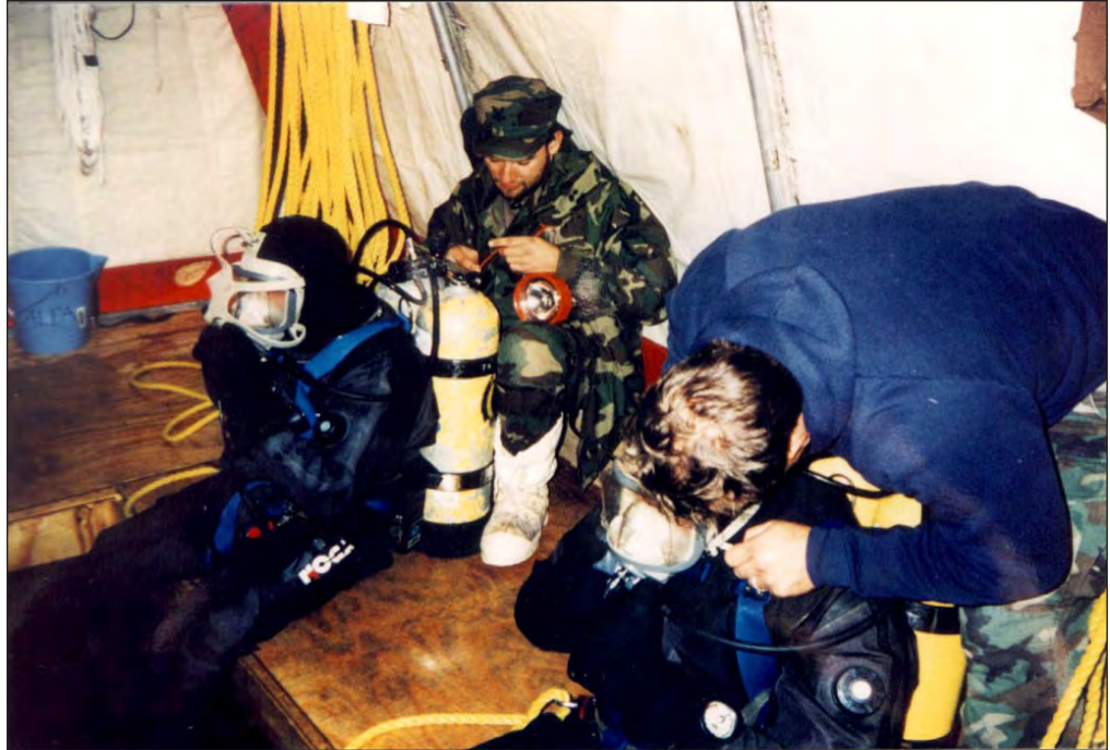
Figure 11-1. Ice Diving with SCUBA. Divers in Typhoon dry suits and Aga/Divator FFM SCUBA with approved cold-water regulators.
