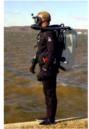
Figure 18-1. MK 16 MOD 1 Closed-Circuit Mixed-Gas UBA.
