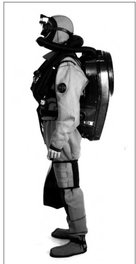
Figure 17-1. MK 16 MOD 0 Closed-Circuit Mixed-Gas UBA.
