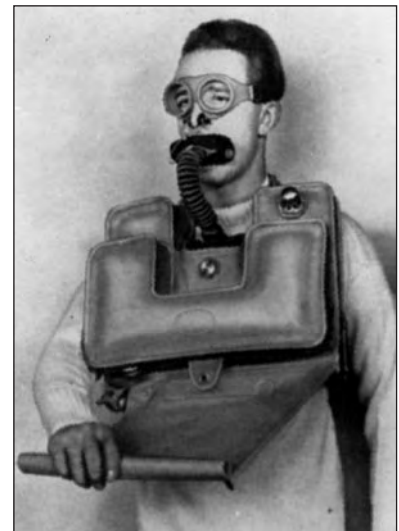
Figure 1-10. Original Davis Submerged Escape Apparatus.
