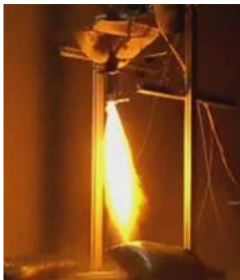
Figure 13 – Testing has demonstrated the functionality of this low cost hydrogen/oxygen thruster (Credit: Innovative Engineering Solutions)
