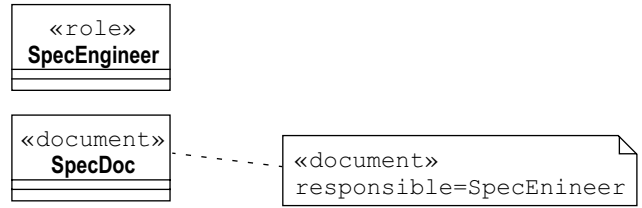
Figure 4: A UML Model That Uses Stereotypes.
