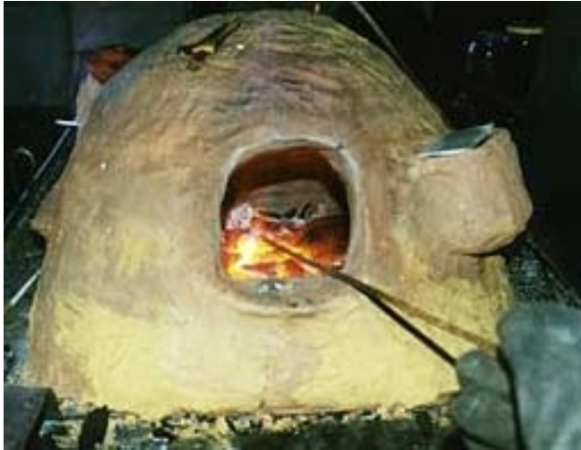
Illustration 5: Small Glass Furnace (Dahlskog and Martensson undated)
