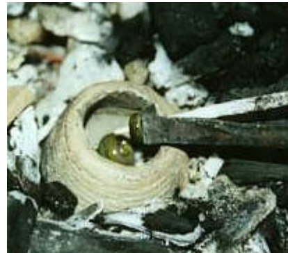
Illustration 8: Annealing Pot (Dahlskog and Martensson undated)
