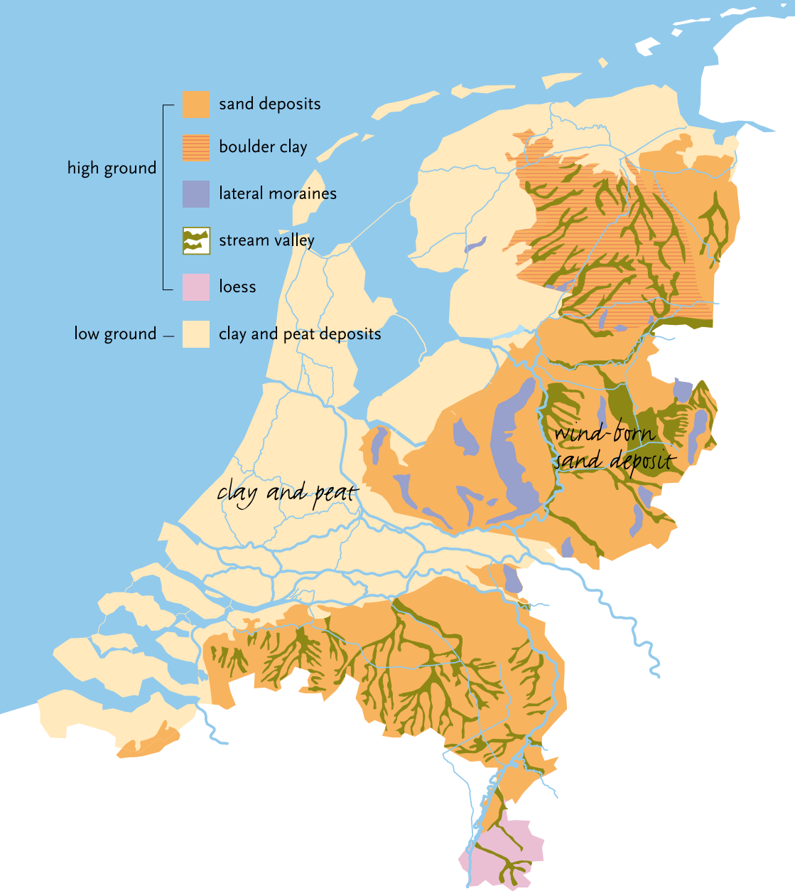
Soil map of the Netherlands: high grounds with wind-borne sand deposits drain into low-lying grounds with Holocene deposits.
