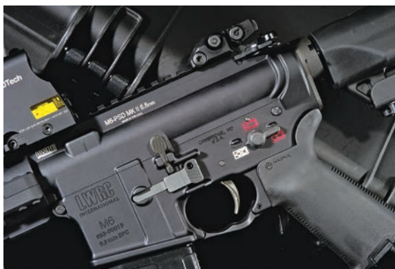
The magazine release is ambidextrous and the trigger guard enlarged for use with gloves. The infinity symbol indicates full-auto has been selected.
