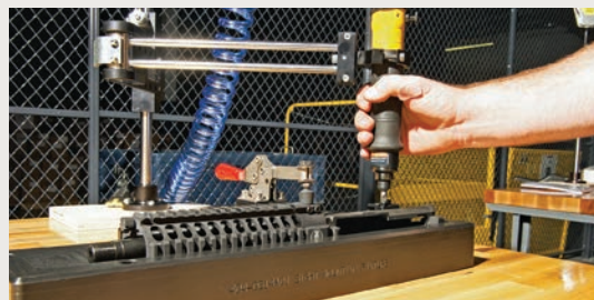
Putting together an AR variant in a factory setting is a lot different than home 'smithing. Torque settings have to be adhered to exactly.
