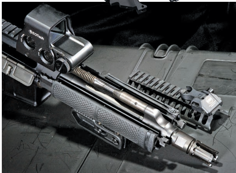
The UCIW SIX8 utilizes LWRCI's patented short-stroke piston design for operation. This reduces both fouling and heat injected into the action.
