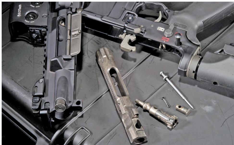
A look at the SIX8's bolt carrier assembly, stripped. Note the rear part of the carrier, which has been modified to help prevent carrier tilt.
