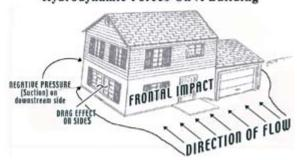
The speed of moving water is called velocity. The faster water moves, the more pressure it puts on a structure and the more it will erode stream banks and scour the earth around a building's foundation.
