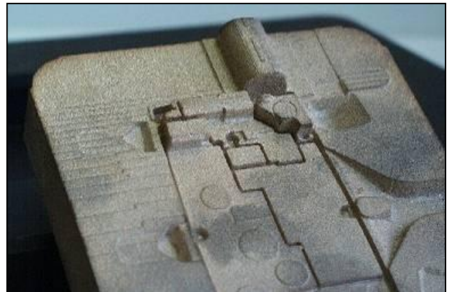
Fig 5 - Rapid Tooling cavity made by ProMetal 3D Printing (Image courtesy of Prof. Richard Hague, Loughborough University UK)
