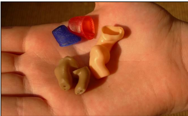
Fig 11 – In the Ear Hearing aids produced by the Envisiontec Perfactory RM process
