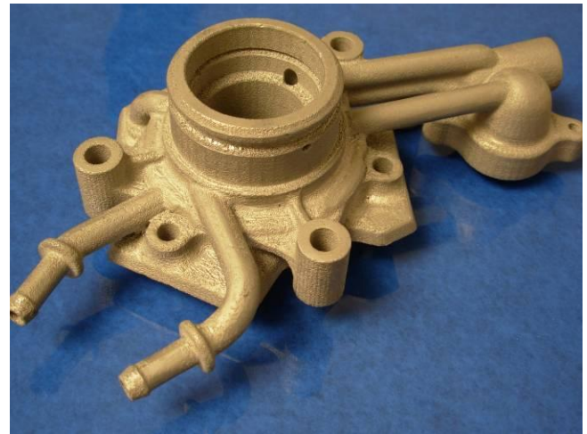
Fig 10 – Selective Laser Melted RM part designed with material optimisation
