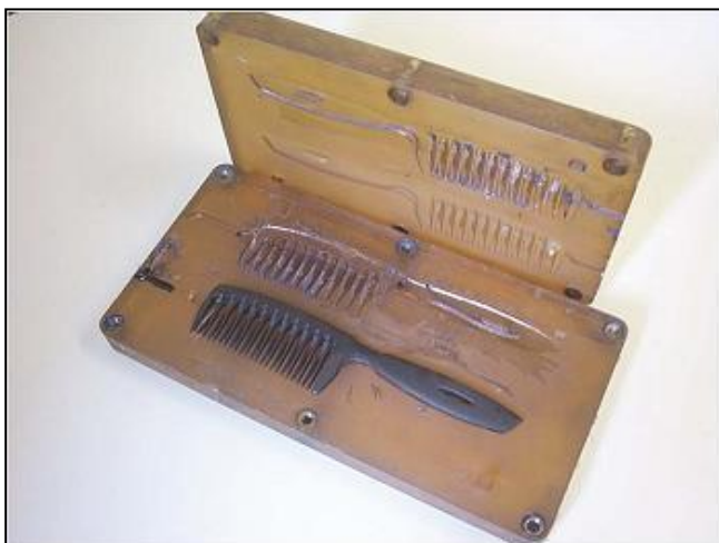
Fig 4 - Stereolithography soft tool cavity (Image courtesy of Prof. Richard Hague, Loughborough University UK)
