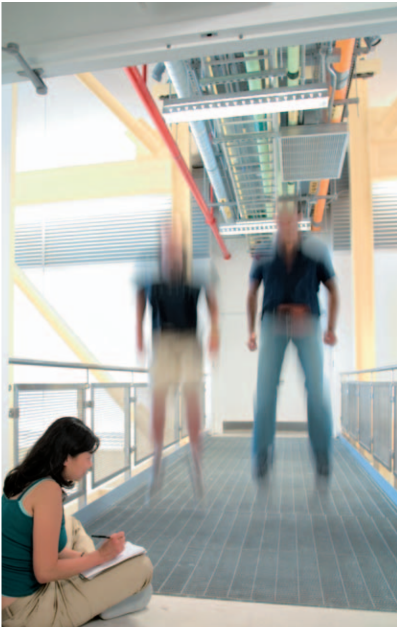
Students measure strain on a Kim Building internal bridge.
