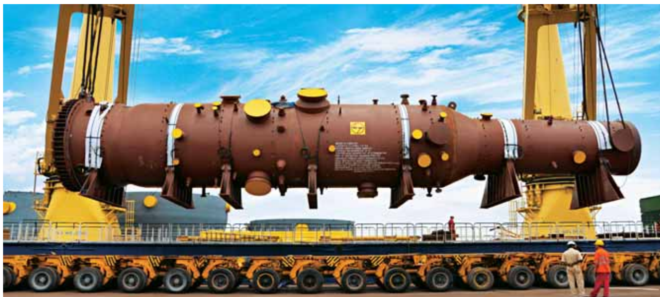
Reactors sail out from L&T's manufacturing facility at Hazira for coal gasification plants in Vietnam.
