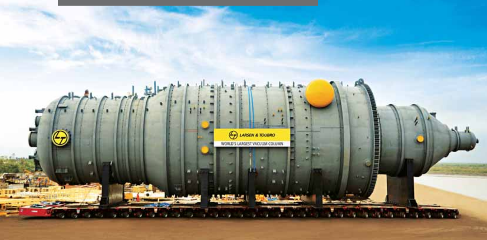
World's largest vacuum distillation column - weighing 975 MT - fabricated by L&T for Paradip refinery (Orissa, India).
