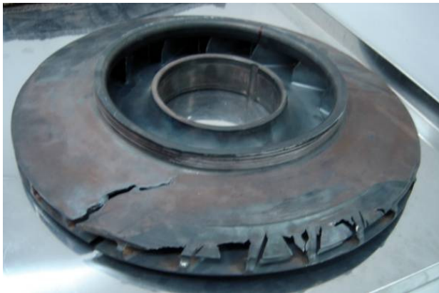
Figure 1. Fracture on Cover
