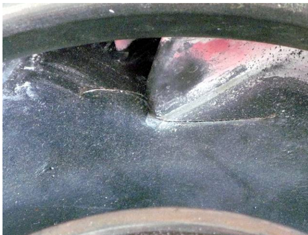
Figure 18. Crack at the Junction of Blade and Disc
