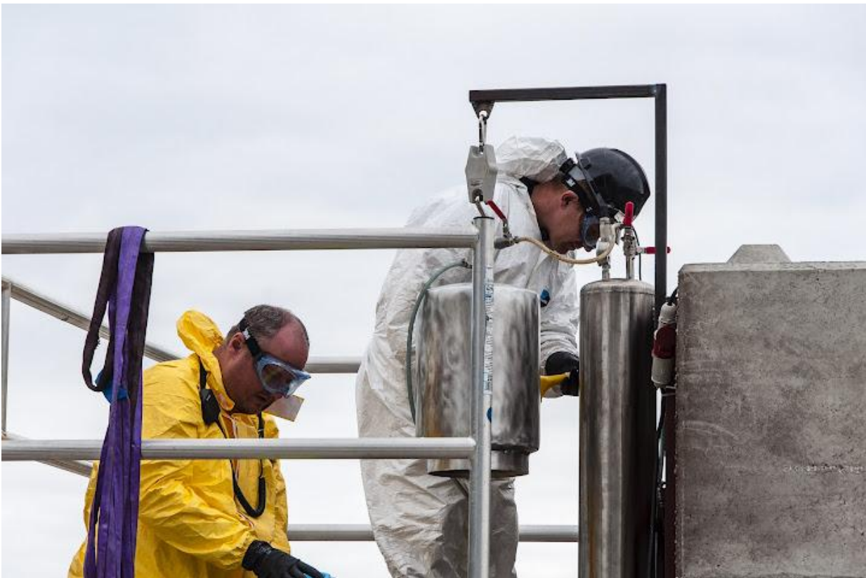
Figure 2 Propellant is loaded. Note storage tank under load cell. Photo: CS
