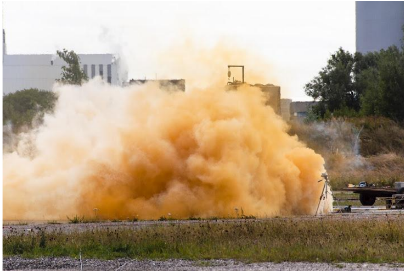
Figure 4 N2O4 fumes formed from the spill of 3 kg WFNA. Photo: CS
