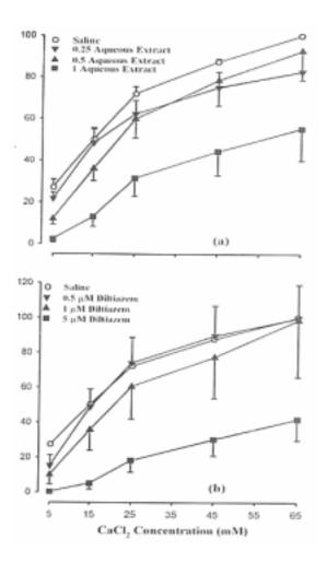
**Figure.** Cumulative concentration-response curves of  $CaCl_2$ -induced contraction of guinea pig tracheal chains in the presence of three increment concentration of aqueous extract from N. sativa (a) and diltiazem (b). Three concentrations of both aqueous extract and diltiazem caused rightward shifts in  $CaCl_2$ -response curves compared to the curves obtained in the presence of saline.
