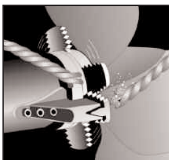
Figure 3. A diagram of an installed line-cutting device depicts the mechanics of how it is intended to function when in operation.
