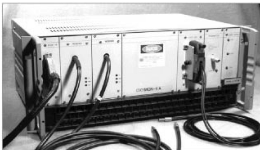
Fig. 5 Near-infrared spectrophotometer (Oxymon, Biomedical Engineering Department, University of Nijmegen, NL) as has been used in this study for the measurement of tissue oxygenation and haemodynamics in human skeletal muscle.
