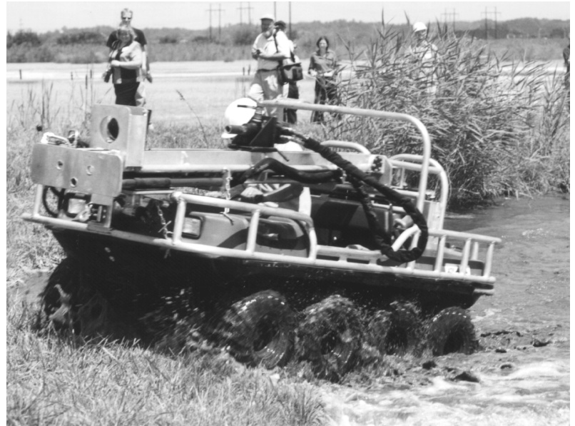
The Argo is an amphibious vehicle, which can travel both on land and into the sludge pond. It should prove invaluable in recovering samples.
