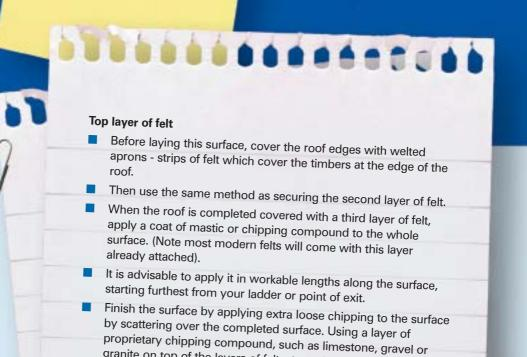
granite on top of the layers of felt, strengthens the surface further. The idea is for the surface to reflect rather than absorb
