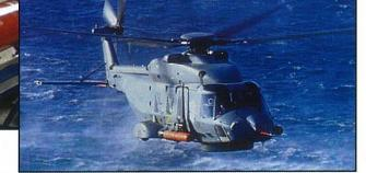
In order to support operational training requirements, a Practice Delivery Torpedo (PDT) is made available to the customers. The PDT is a non-propelled version of the MU90 torpedo and is aimed to allow low-cost training for the personnel.
