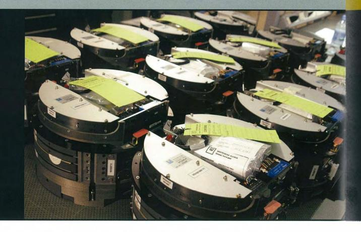
The MU90 / IMPACT torpedo is an electricallypropelled weapon. It is powered through an Aluminium-Silver Oxide (AgO-Al) sea water battery using dissolved sodium-dioxide powder as electrolyte.
