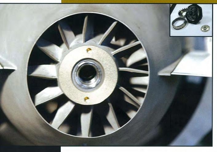
The MU90 / IMPACT torpedo is propelled through an electronically controlled high-RPM brush-less motor housed into the torpedo through antivibration mountings.
