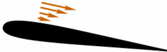
Figure 10. The variation of the speed of a fluid near an object
