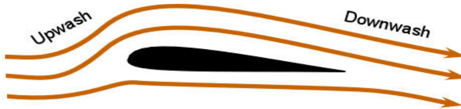
Figure 5. True airflow over a wing with lift showing upwash and downwash.
