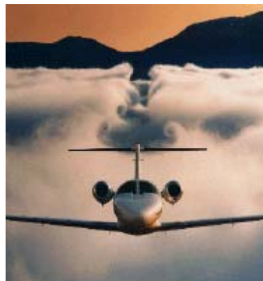
Figure 7. Downwash and wing vortices in the fog.
