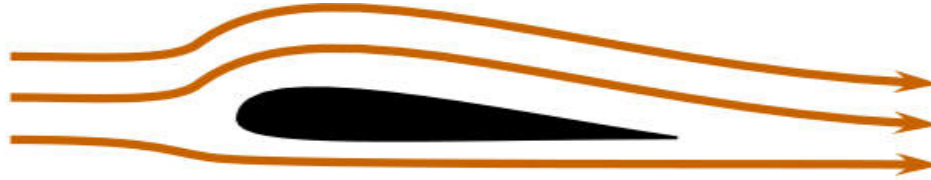
Figure 4. Common depiction of airflow over a wing. This wing has no lift.
