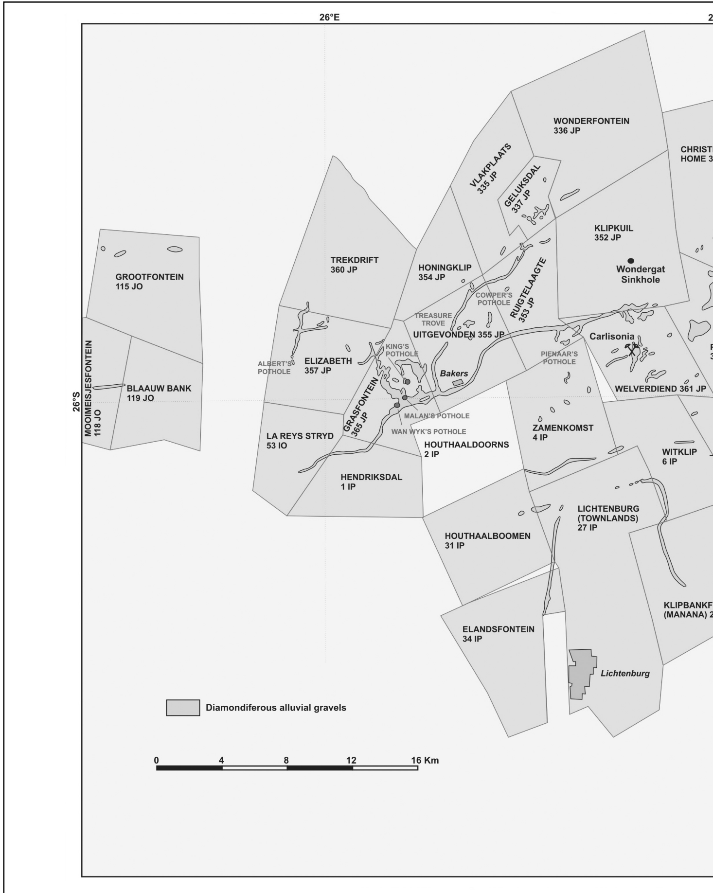
Figure 5. Plan showing the known diamondiferous alluvial gravels around Lichtenburg, modified after Du Toit (1951).
