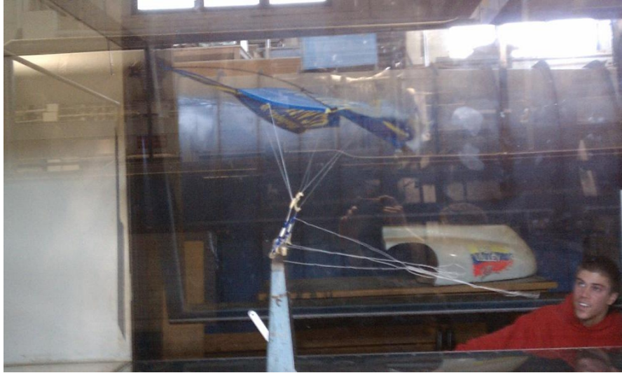
Figure 9: Mostly stable flight at 18 degree angle
