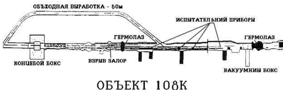
Figure 13. Plan view of tunnel 108k, Degelen test site. It was at this site that a nuclear device was left sealed underground, when the Russians abandoned the test site in the early 1990s. In 1995, the device was destroyed in place by a 30 kg high-explosive charge.
