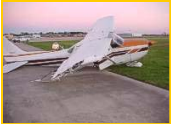
A damaged C-172 after midair with a C-150. The C-150 crashed killing its pilot, the sole occupant. The two on-board the C-171 were unhurt.
