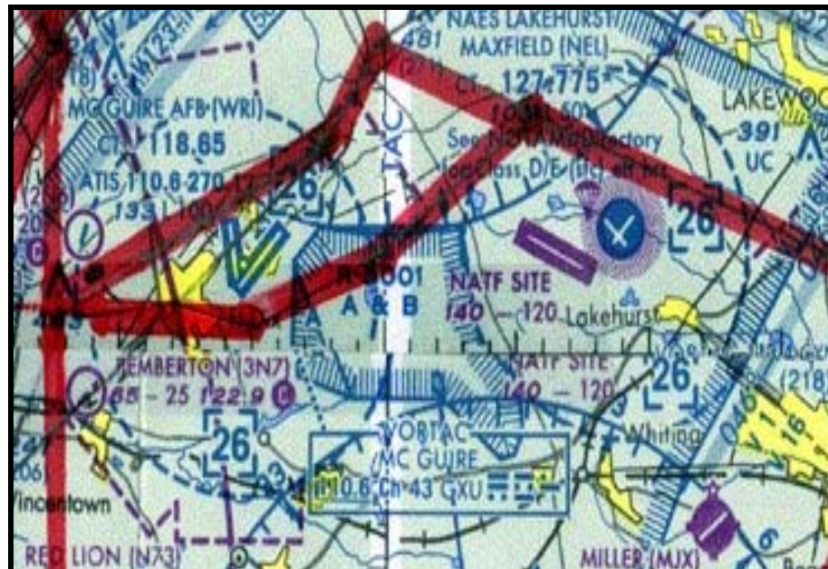
Sectional depiction of Class D airspace of McGuire and Lakehurst, note Class E extensions off McGuire's Class D (not to be used for navigation)
