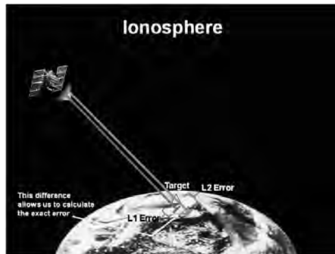
Figure 16-4. Error induced on L2 by the ionosphere. (NSSI graphic prepared by the author)
