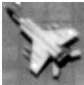
Figure 13-1. 48-inch GSD. (Reprinted from Jeffrey J. Hemphill, "ITEK Optical Reconnaissance Camera System: Comparing Resolution and Area Coverage," http://www.geog.ucsb.edu/~jeff/115a/militaryintelligence/itek.html [accessed 5 April 2008].)
