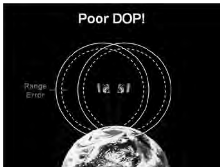
Figure 16-5. Poor constellation geometry or DOP. (NSSI graphic prepared by the author)
