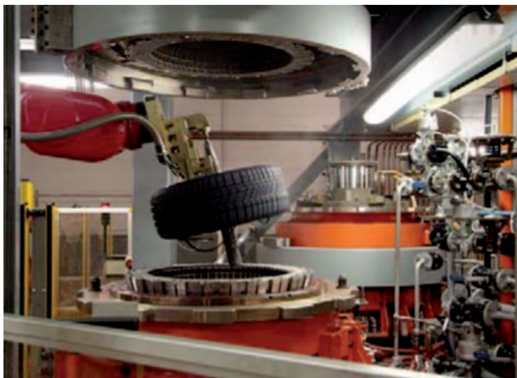
(LEFT) THE MIRS™ VULCANISATION PROCESS (RIGHT) TYRES COMING OFF THE PRODUCTION LINE
